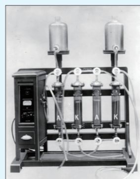
Heat-free water distillation system
